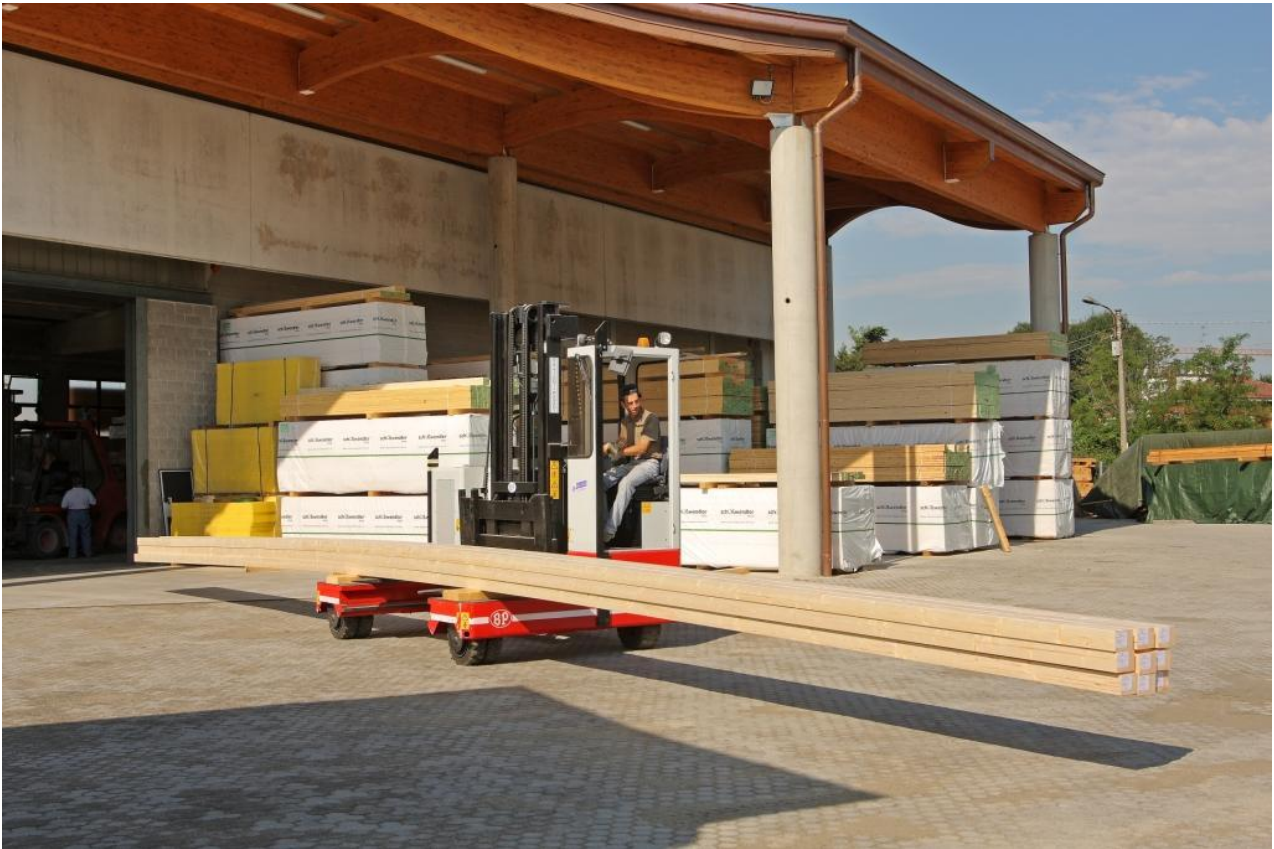
ML-T4: 4 ton electronic computer drive multidirectional forklift operating at a indoor and outdoor wood panels warehouse
