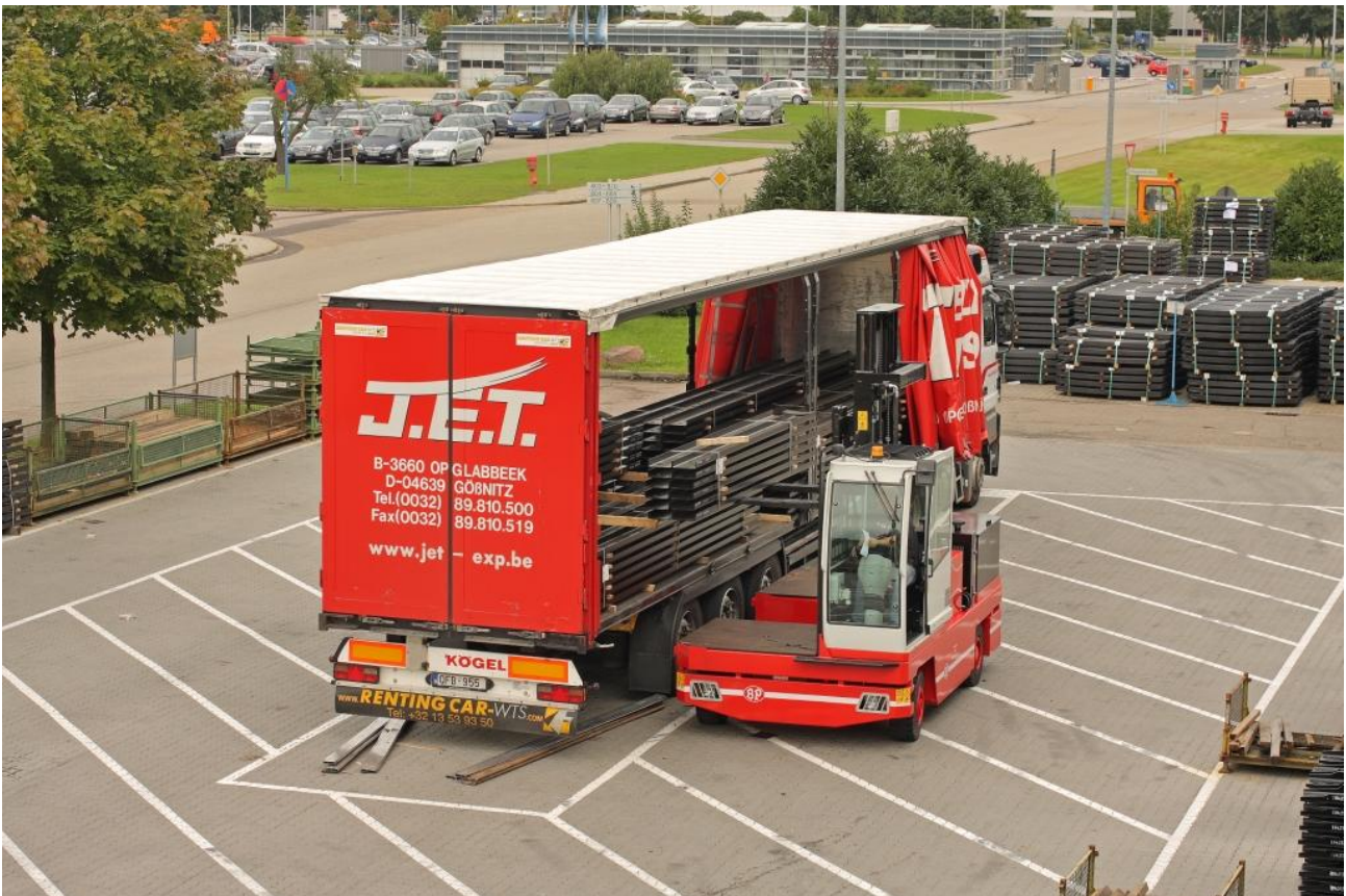
HT5EL: 5 ton electric AC side loader loading steel frames on truck at a logistic warehouse site
