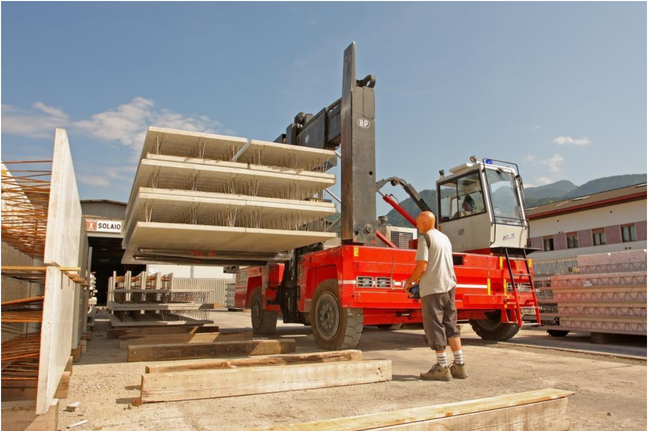
HT20: fully remote controlled 20 ton side loader equipped with telescopic hydraulically tunable beam handling concrete bars
